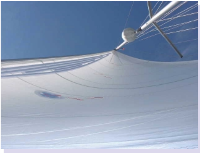
Here the sail is completely unfurled, the amount of shape (camber) is represented numerically and is 16% in the mid-section and 16.7% in the top section.
