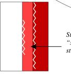
Staggered tape finishing eliminates "stacking" of stitching and produces a stronger, smoother edge.
