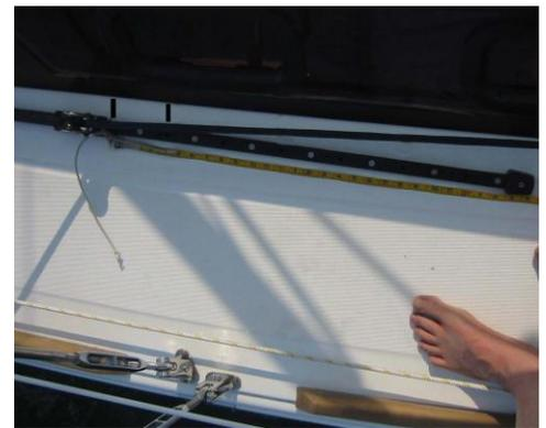
*Car location when reefed to the reef 1 mark. Note both marks on the deck for full size and reef 1*
